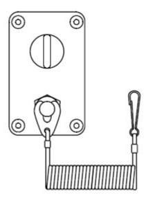
The engine will not run without the plastic clip on the **Engine Safety Lanyard** attached to the safety switch. The spring loaded safety switch is integrated with the ignition switch. If the clip is removed from the switch while the engine is running, the engine will shut down.
