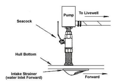
Note: If the seacock is left open, the forward motion of the boat can gradually fill the livewell tank even when the livewell pump is not turned on.
