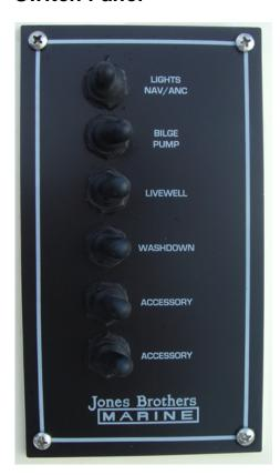
The switch panel is located on the console and has six toggle switches. In the picture on the left, all switches are in the OFF position - the lights switch is in the middle position and the remaining switches are thrown to the right.
